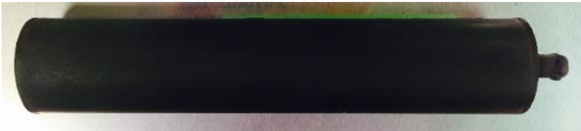
Figure 3.47 Metallic capsule of 2" diameter and 10" height (with Rust-Oleum coating)
