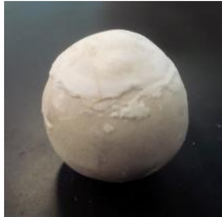
Figure 3.39 Capsule that survived 510 thermal cycles
