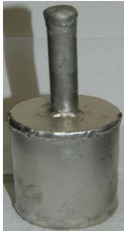
Figure 3.46 Ni coated carbon steel capsule
