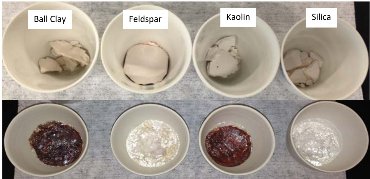
Figure 3.15 Components of ceramic mixture sintered at 800°C (top) and subsequent treatment of the sintered components with molten sodium chloride at 850°C for 24 hrs (bottom)
