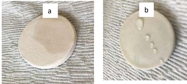
Figure 3.11 a) Hydrophilic, sintered at 800°C b) hydrophobic, sintered at 1190°C
