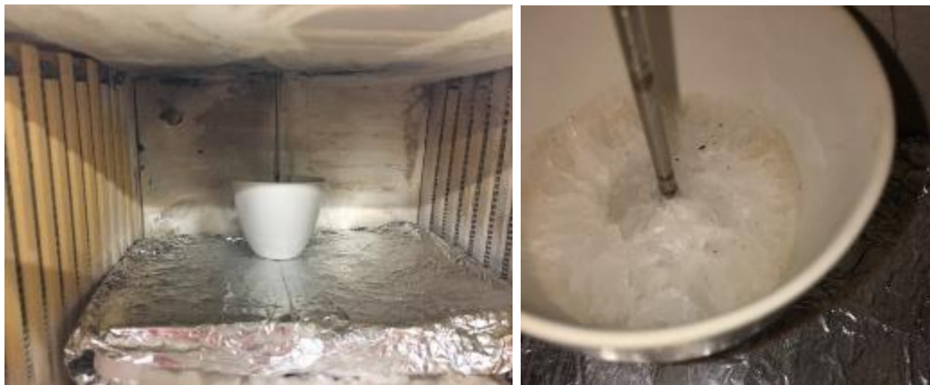
Figure 3.26 Solidified bottom layer with the attached thermocouple
