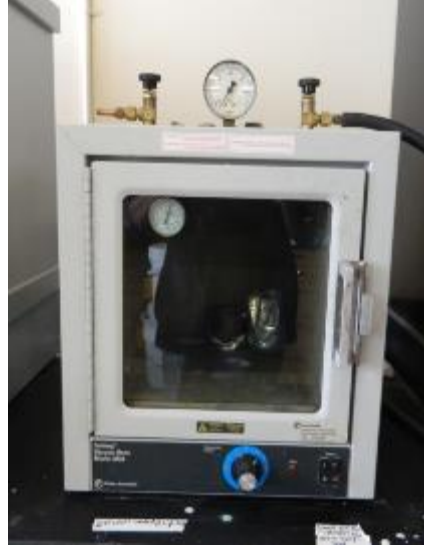
Figure 3.5 Vacuum furnace (Isotemp 280A)
