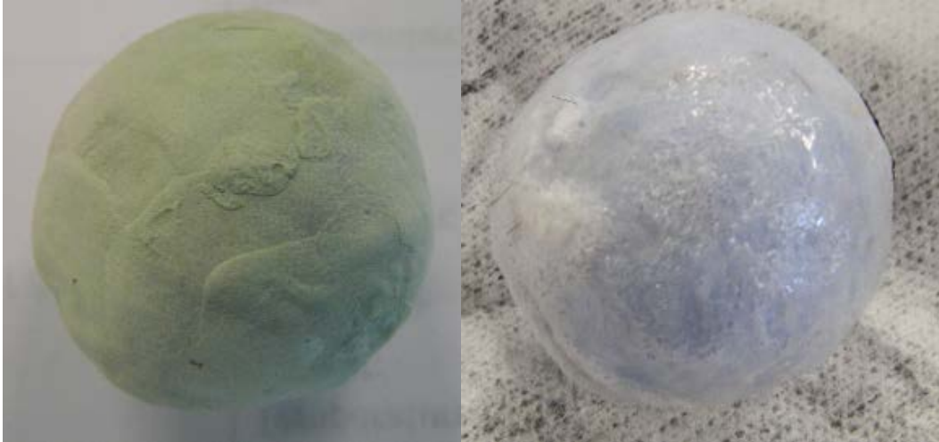
Figure 3.19 Ceramic coated sodium chloride salt pellets
