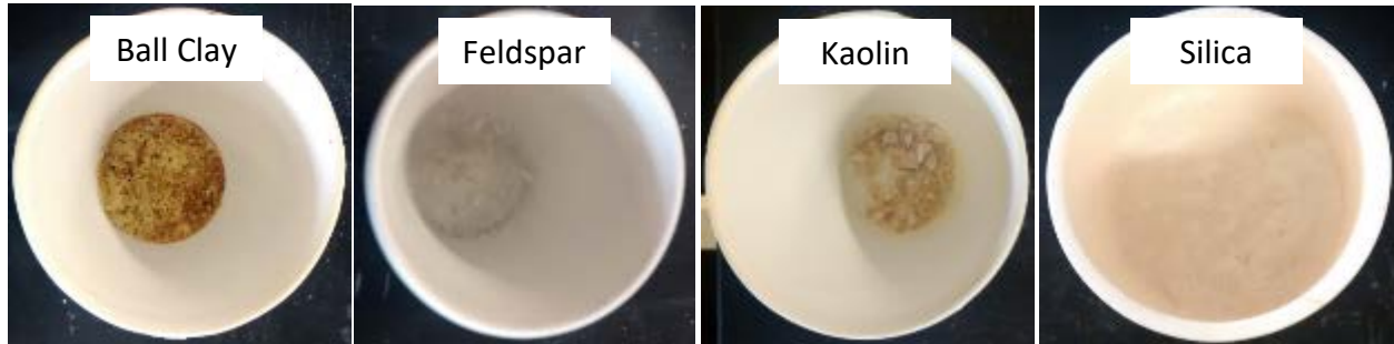
Figure 3.17 Sintered (1190 °C) ceramics after treatment with molten NaCl at 850 °C for 24 hrs
