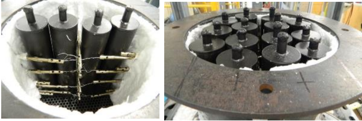
Figure 4.4 Capsule arrangement inside the storage tank
