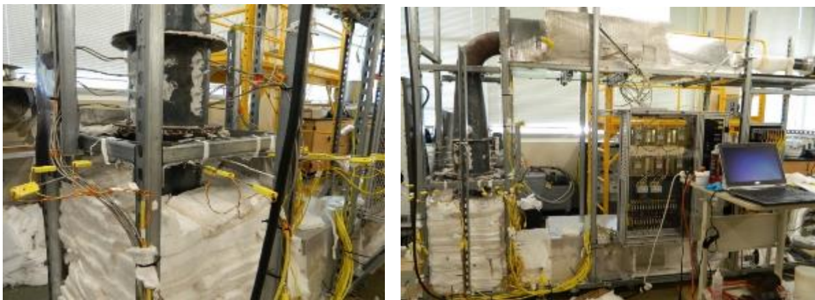
Figure 4.5 Storage tank with the thermocouples (without the insulation)
