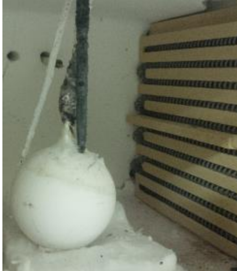
Figure 3.25 Corrosion of thermocouples (investigation of melting for an enclosed spherical capsule)
